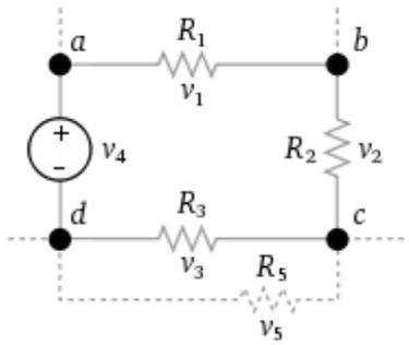
The sum of all the voltages around a loop is equal to zero.
