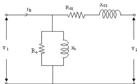
**EQUIVALENT CIRCUIT FOR OC AND SC TEST**
