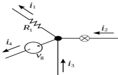
The current entering any junction is equal to the current leaving that junction.  $i_2 + i_3 = i_1 + i_4$
